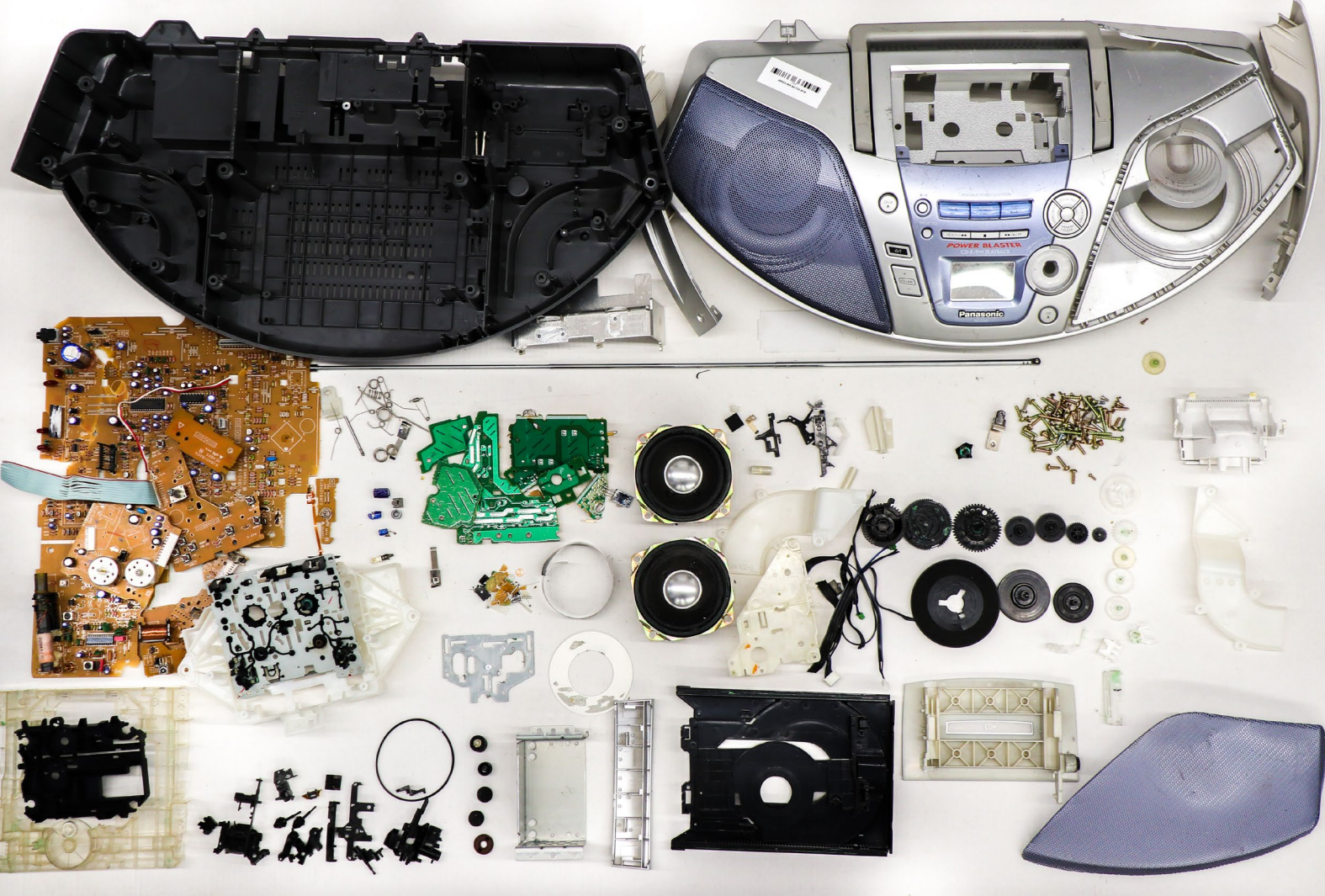
Figure 3: Finely dismantled boom box.
